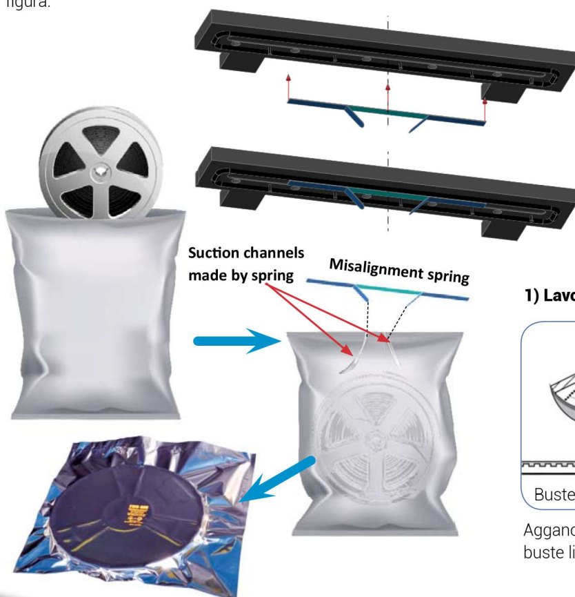
Figure 3-1 Typical Dry-Pack Configuration for Moisture-Sensitive SMD Packages in Shipping Tubes
