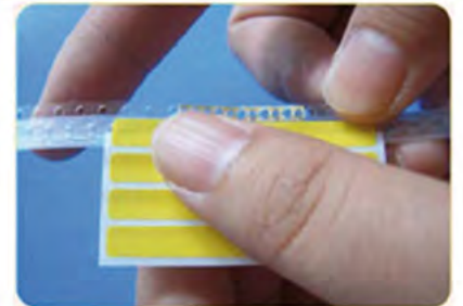
Step 6: Black strip in line with the edge of the reel to stick splice tape.
